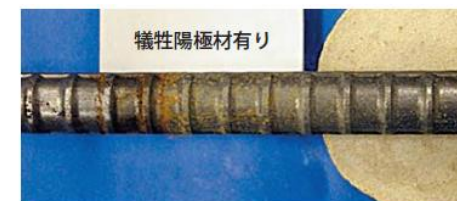
鉄筋腐食促進試験 Accelerated Corrosion Test
