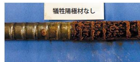
鉄筋腐食促進試験 Accelerated Corrosion Test
